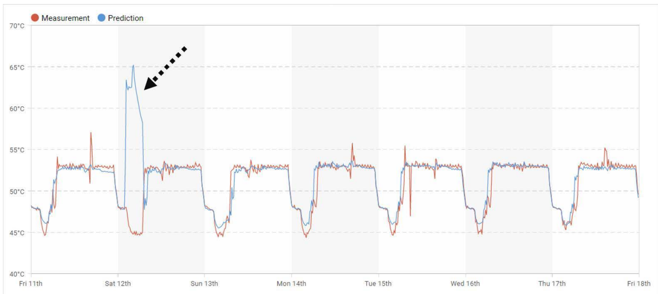
Figure 3. Measured and predicted temperature of domestic hot water. On Saturday morning (the black arrow), one can see an expected rise in temperature due to Legionella prevention; however, there was no rise in the measured temperature profile (red line) due to the wrong schedule setup.
