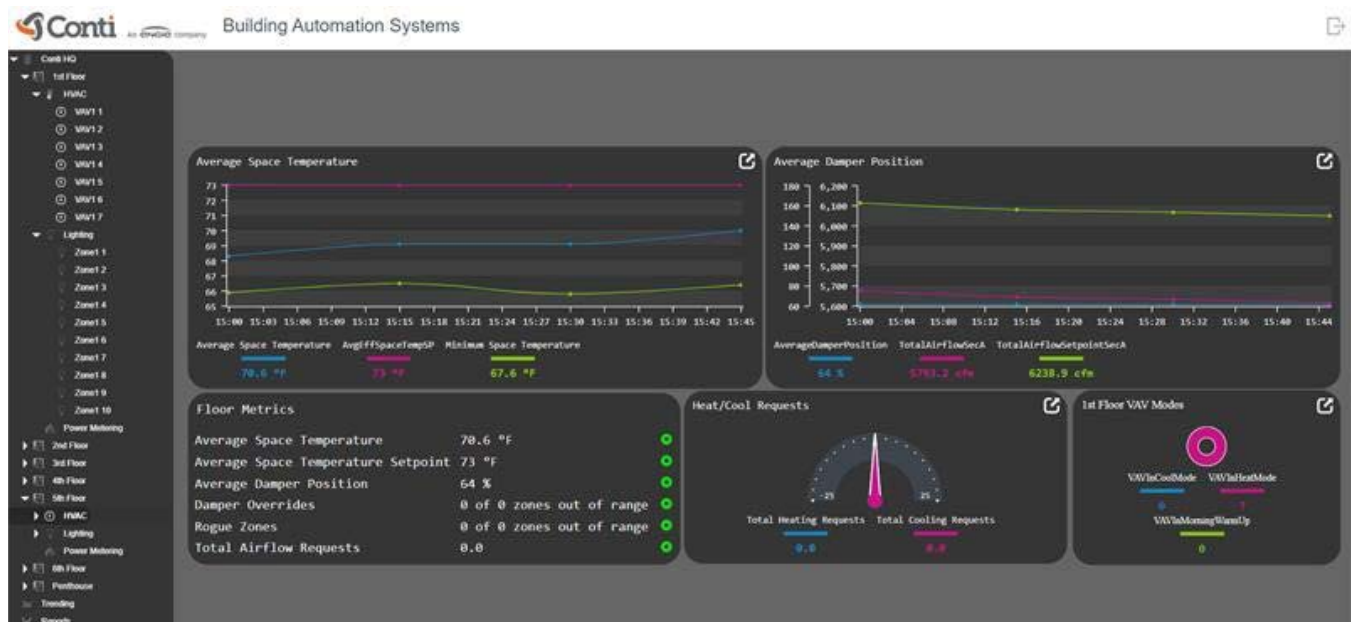
Figure 1. Floor-level metrics allow a secondary evaluation of floor-level conditions, easily identifying any deficiencies in floor-level units or the upstream units serving the floor. From one graphical page, the end user can determine mode, operation and operator overrides that could negatively influence the space.
